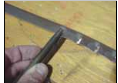
First form one side of the crimp, then twist the handle the other way.
