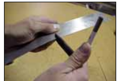
Twist the handle first one way, then form the other half of the crimp
