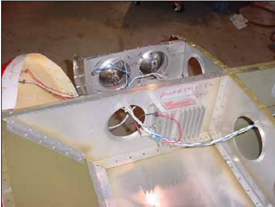
Installation of the drive unit for the strobe lights, Ref option drawing 6-NSO-1
