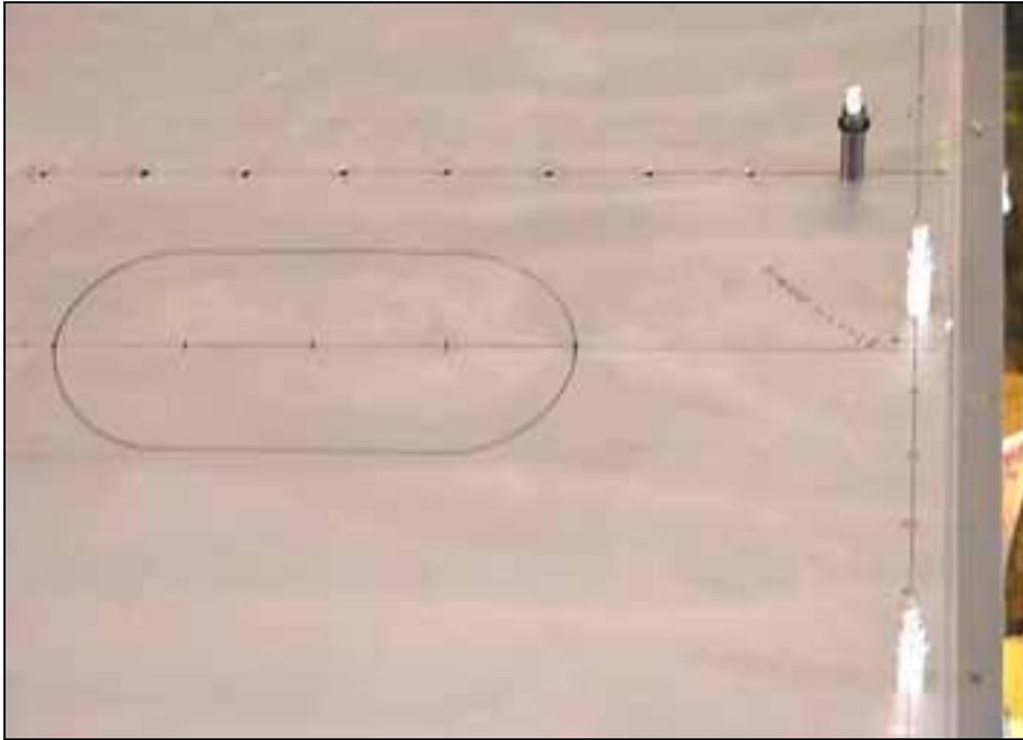
Access hole for the aileron bellcrank is on the O/B side of RR#7
