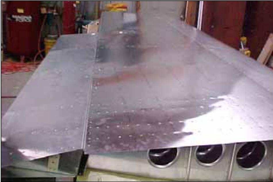
Drill the aft rivet line through the Piano hinge.
