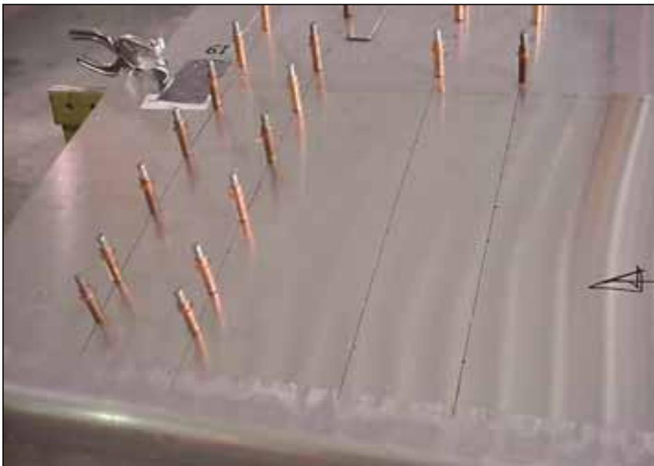
Layout: Mark the span-wise rivet line 10mm from the aft edge of the Bottom Spar Cap Angle 6W3-7. Divide the distance between the intersections A5 pitch 40. 3 rivets pitch 20 on each side of rib #9. Layout the rivet pitch through the nose rib.
