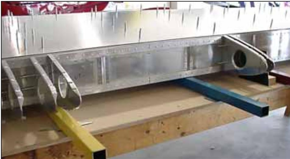
TIP: Position the wing assembly on the workbench with the front of the nose ribs over the edge of the workbench.
