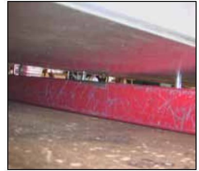
Note the visible gap between the top of the beam at rear rib #9 and the bottom skin.
