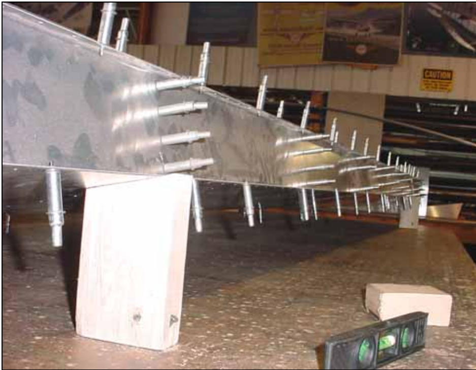
Check that the rear channel is level.
