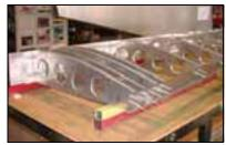
Check: Sight down the rear channel 6W7-1 and the spar, check that they are straight. The aft edge of the channel is the reference to position the Rear skins.
