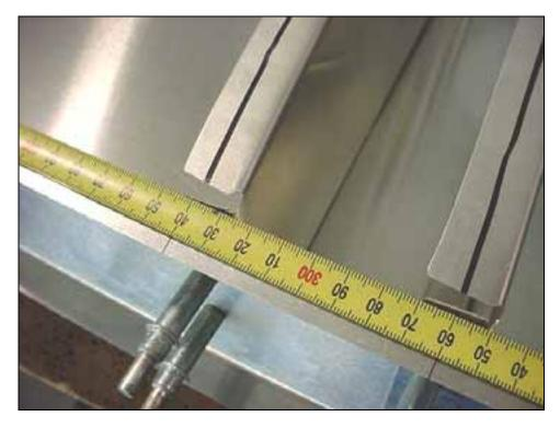
Layout & mark the rib stations along the aft edge of the of the rear channel, Ref 6-W-7  $\,$
