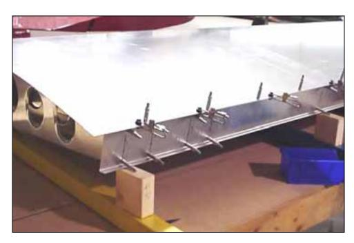
Start drilling along the aft edge into the top flange of the Rear Channel.
