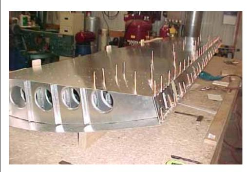
First drill through the rear channel. Drill from the back moving forwards.
