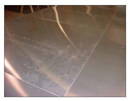
Orientation: the pre-drilled holes are along the <u>aft</u> edge of the rear top skin 6W8-3.
