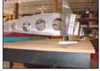
If necessary, add spacers between the workbench and the beam to level the spar.
