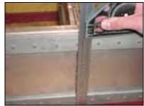
Mark the rib station along the top of the spar.
