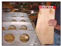
Use plywood template shown on drawing 6-B-14. Also refer to photo assembly section 6-B-11A.
