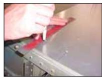
Also extend the rib rivet line to the front edge of the skin.
