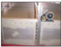
Note: the ribs stations shown on drawing 6-W-3 does not always correspond to the center line of the rib flange. Refer to drawing for the flange orientations.
