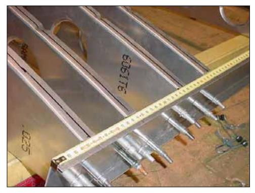
Layout the ribs stations along the aft edge of the top flange of the rear channel 6W7-1. Hook the end of the tape measure on the I/B end of the channel and layout the rib stations as shown on the middle diagram on drawing 6-W-7.
