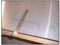
Also mark the rib stations along the front edge of the skin. Use a straight edge to extend the pre-drilled line to the edge of the skin.
