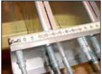
Mark the ribs station on the aft edge of the flange.
