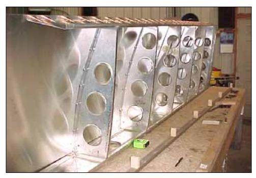
The tack rivets keep the wing skeleton from shifting as the wing is turned over.
