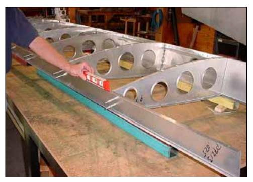
Position the beam (support block) underneath the rear channel to keep the main spar level and at 9 degrees.
