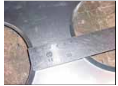
Layout the midpoint between the lightening holes.
