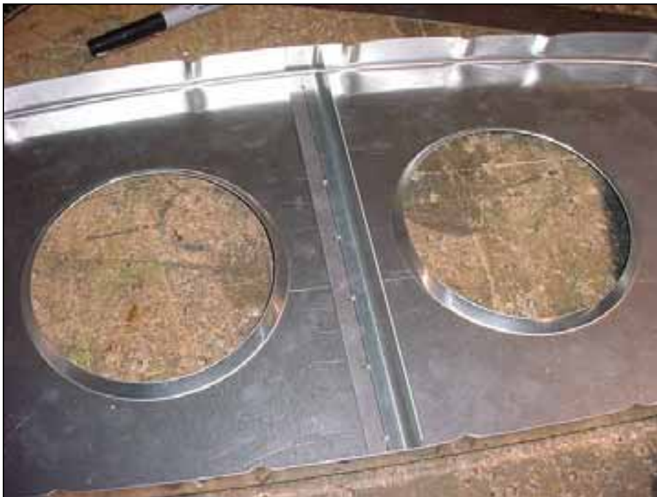
Pre-drill the L angles with #40 pilot holes.
