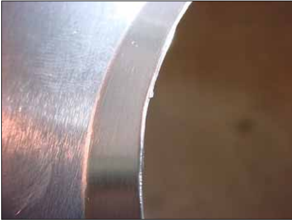
Burr on edge of flanged lightening hole.
