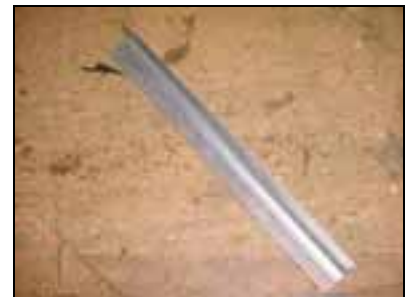
Pre-drill the L angles with #40 pilot holes.
