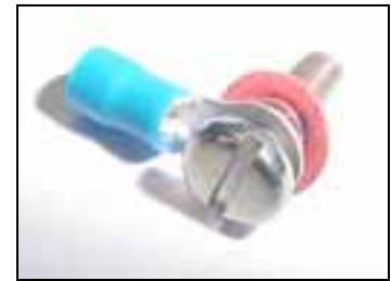
Ring terminal (ground) over paper washer.
