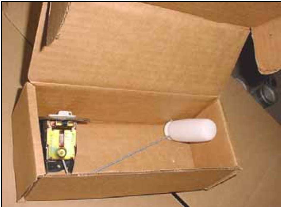
Float type fuel sender unit in supplier box. Use VDO Fuel Level Gauge 70-10 Ohms; turn to last page of this section.
