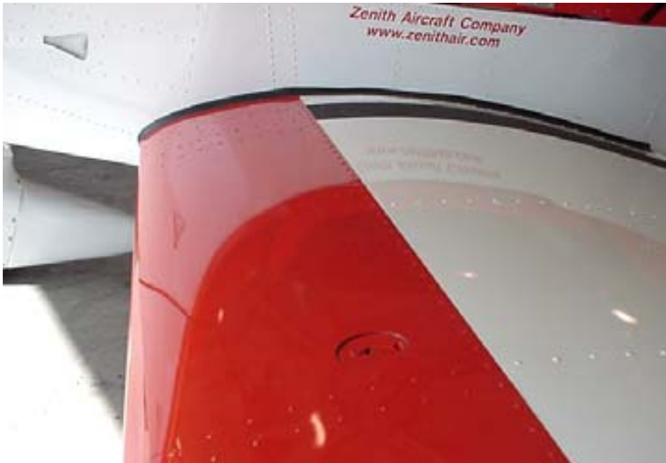
LE Tanks Installed on the front side of the spar between NR #4 & #5
