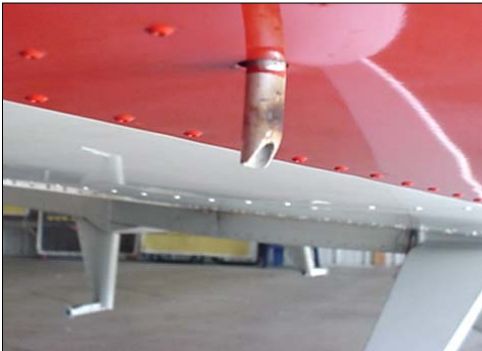
Hole in the bottom of the Leading Edge Skin for the Vent tube
