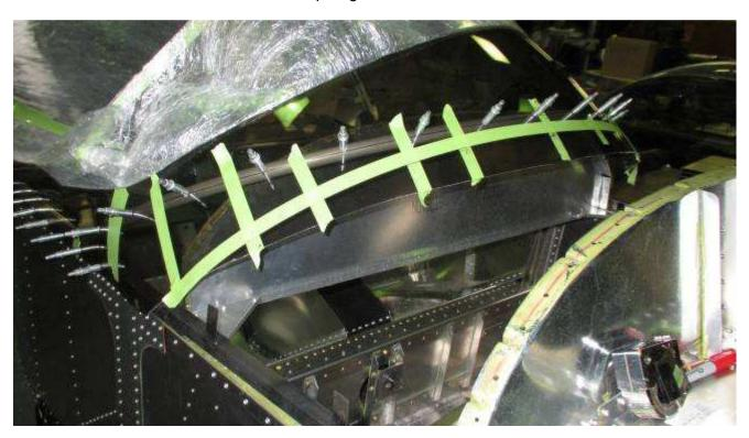
Sight across the firewall and instrument panel to make a mark on the piece of tape. Use a flexible edge to connect the points and trim.
