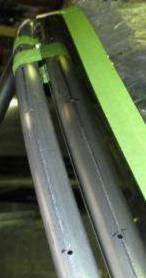
Position the front canopy on the fuselage. Line up the aft edge between the 2 tubes.
