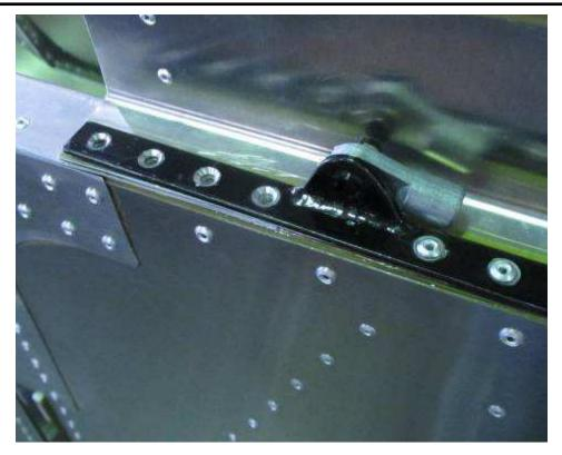
Countersunk holes in the aft portion of the bottom bracket 65C2-2
