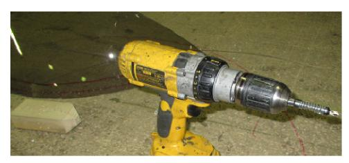
IMPORTANT: Use a wood block on the back-side to drill a clean, shatter-free hole.
