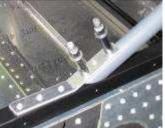
Remove the bubble to rivet the brackets to the side tubes.
