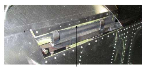
To prevent the welded rod on the canopy side frame from catching and damaging the flange, add rivets in the middle as well as at the ends.
