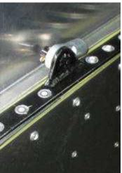
Remember to install the eye 9426K94 before riveting
