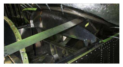
Keep trimming the front edge until it does not touch the strip.
