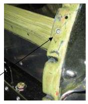
Flush rivet at front through firewall flange
