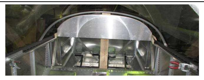
Check that the tube is centered over the instrument panel (left and right sides are equal)
