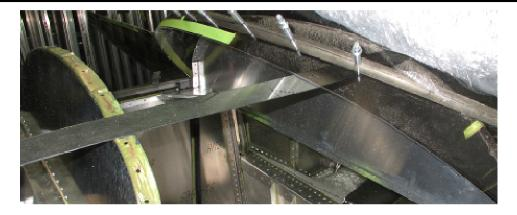
Flexible edge between instrument panel and firewall.
