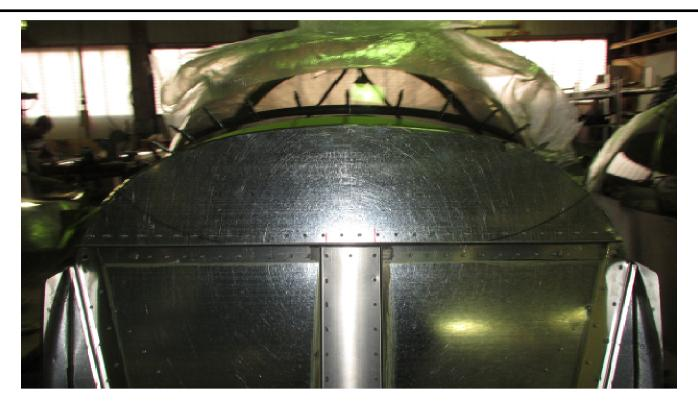
Remove the tube and drill the holes in the plexiglass.
