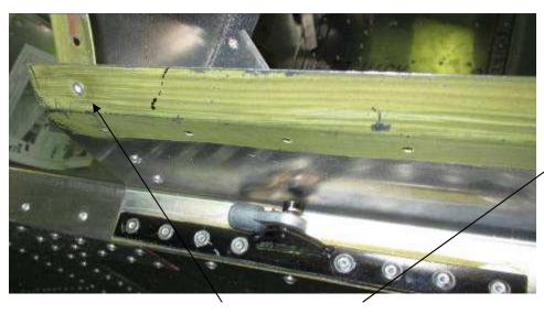
Flush rivets through the instrument panel and firewall.
