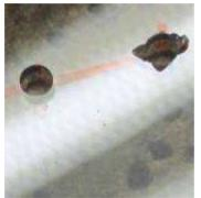
Drill shatter free holes (the shatter is generally located on the back side of the hole)
