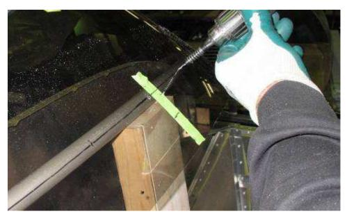
Using the drill to mark the holes with a shallow dimple.
