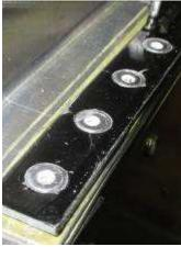
4 flush rivets in the rear portion.
