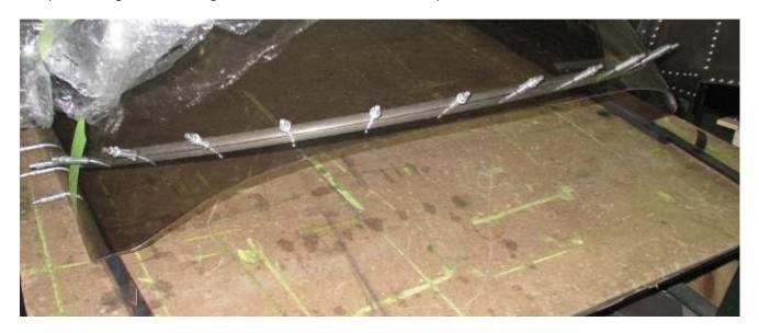
Mark the aft edge of the FRONT CANOPY FRAME GUSSET 65C3-12 on the side frame (left and right side.
