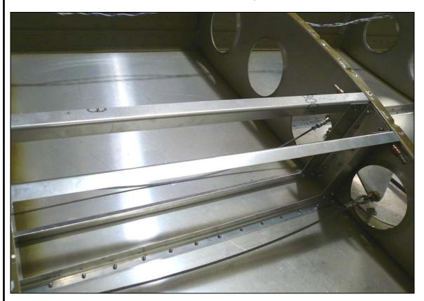
Position the L Angles on flush with the top of the Rear Rib next to the Support Channel and clamp the other end of the L Angle to the Rear Rib top flange. Mark the edge of the Support Channel and layout 2 rivet locations as before. Back drill through the L Angles into the Support Channel and Cleco. Expand the holes with a #20 drill bit.
