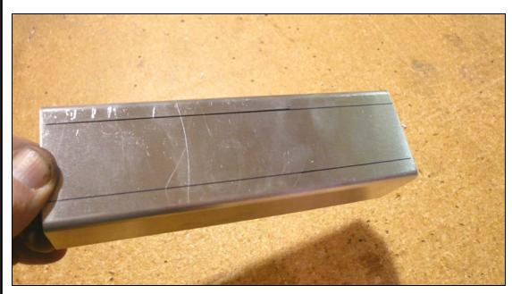
**P/N:** 6ZU3-1 Bellcrank Support Channel
