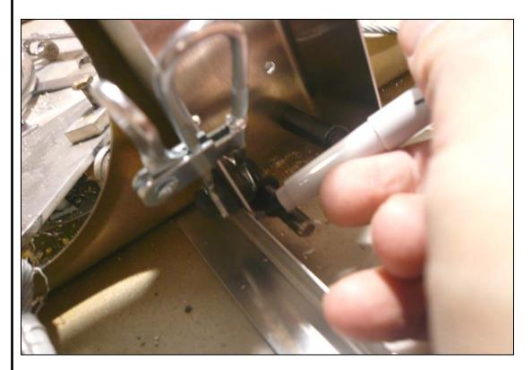
Cut four pieces of L Angle to fit between the Rear Ribs. Position the L Angle at the bottom of the Support Channel on the Bottom Skin. Clamp the L Angle in place. Mark the edge of the Support Channel on the L Angle.
