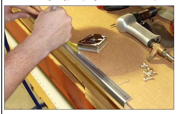
Cut an L Angle to fit between the Rear Rib #4 and Rear Rib #5. If the Wing Locker Option is installed, move on to Rear Ribs #5 and Rear Rib #6. Draw a center line on one flange of the L Angle. Mark a rivet location 10mm from each end and evenly space rivets at approximately pitch 100mm. Use a #40 drill bit to drill the rivet locations.
