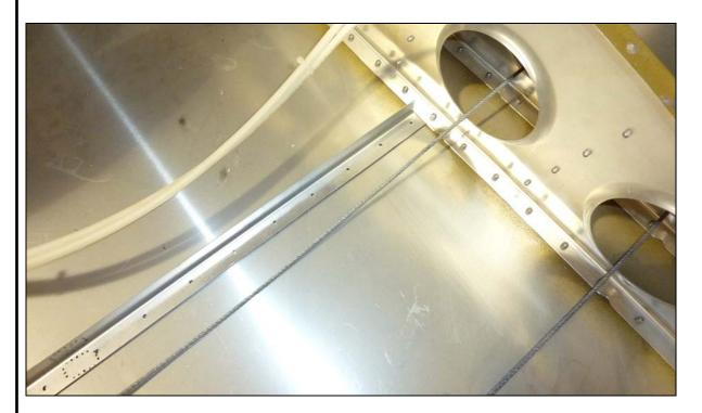
The L Angles installed on the Skins are positioned half way between the Spar and Rear Channel. Measure from the Spar rivet line aft 435mm next to Rear Rib #4 and place a mark on the skin. At Rear Rib #5 measure from the Spar rivet line aft 422mm and place a mark. Draw a line on the Skin at the marks. Position the L Angle with the line visible through the holes in the L Angle. Back drill through the L Angle into the Skin and Cleco. (The L Angle was installed with pitch 40mm in the above photo.)
