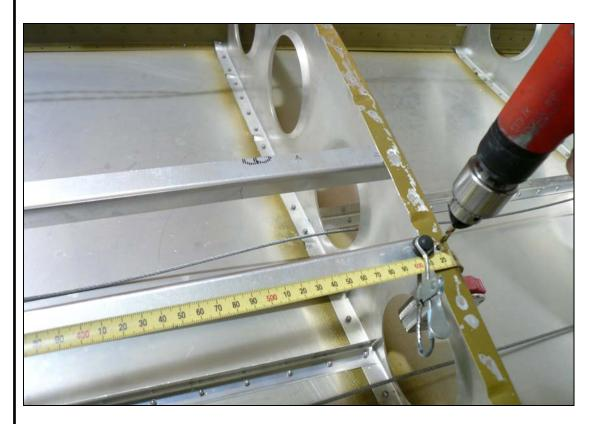
Set the spacing between Rear Rib #6 and Rear Rib #7 to match the Top Wing Skin. Use a #20 drill bit to back drill through Rear Rib #6 into the L Angle and Cleco. (The above photo was taken on the Left Wing as the rest were of the Right Wing.) The top flanges will be drilled when the Top Skin is reinstalled.
