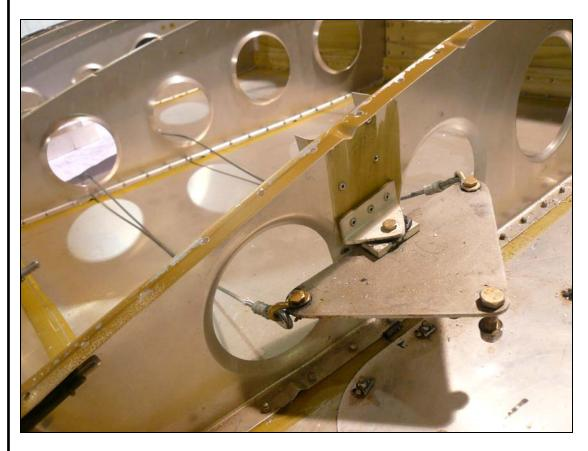
Remove the Aileron Bellcrank and drill out the rivets attaching the Aileron Bellcrank Supports and Bellcrank Support Channel to the Rear Rib.
