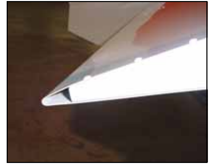
Gap between end of rib and trailing edge is generally left open.
