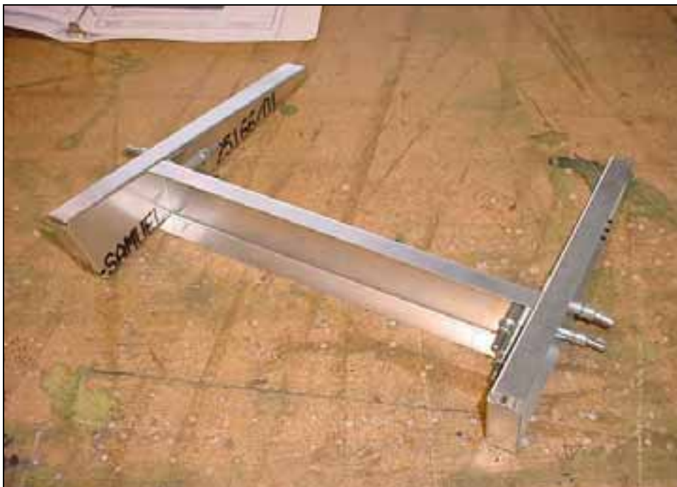
2 RIVETS A5 6T3-2 to "L" angle
