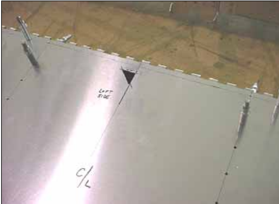
TOP 22mm from front edge of skin (behind the top flange)
