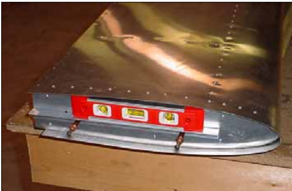
Position a level on extrusion (right side). Shim the stabilizer to center bubble.
