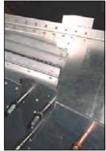
Trim the aft corner of the rear bracket 6B1-8 to make room for the bottom side of the stabilizer skin.
