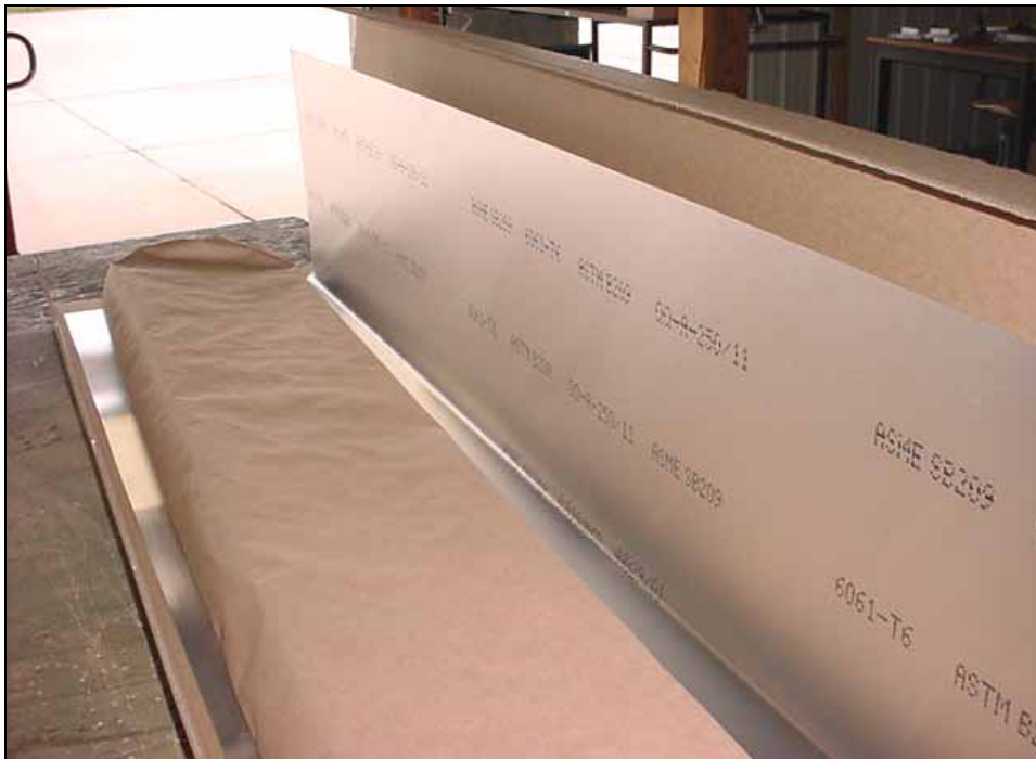
Hold the top of the box with one hand, cut all the pieces of tape, and slowly open the box. The Elevator skin is wrapped in paper.
