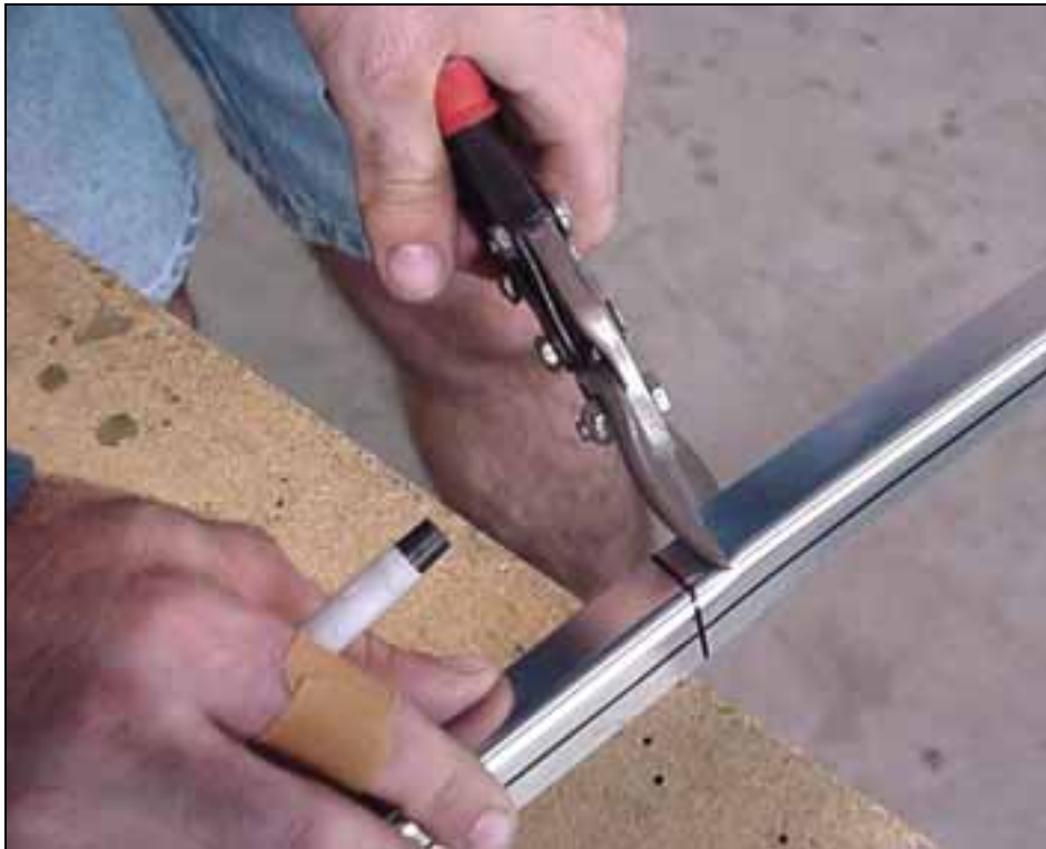
Cutting the “L” angle: Qty = 4 Layout: length = approximately 75mm. Rough cut: Snip both flange, twist to break off. Then do a final cut on the line.
