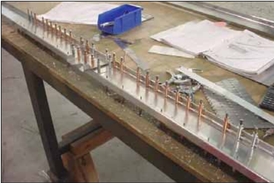
Rear spar with doubler and rear spar attachment.
