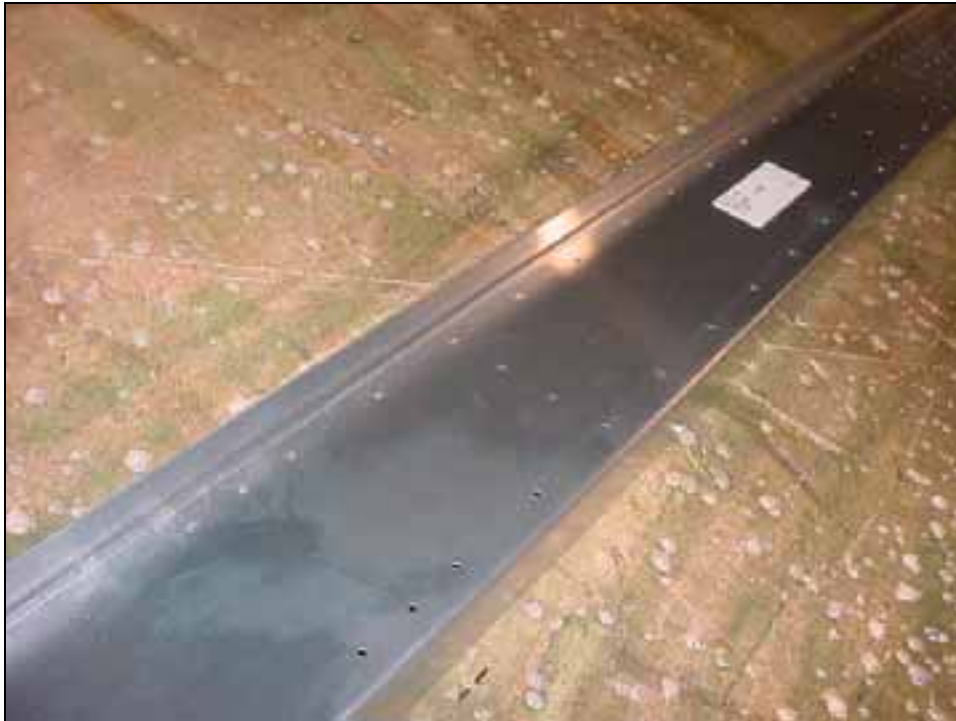
REAR SPAR 6T1-4 (pre-drilled)
