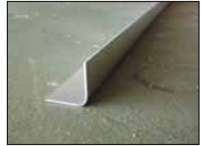
Rear spar upper doubler 6T1-6HD is bent 5 degrees closed.
