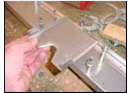
Layout the center line on the rear spar attachment 6T2-3.
