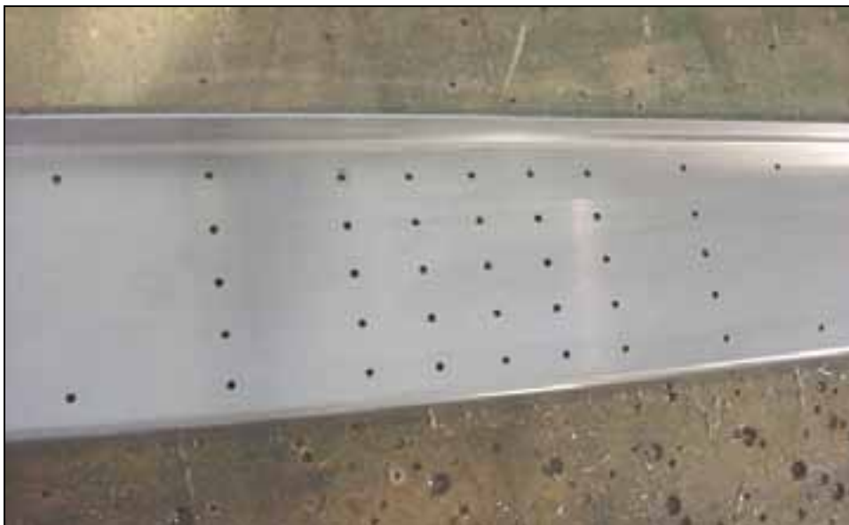
Rivet lines at the end of the shim 6T3-6HD 15 holes = rear spar attachment 6T2-3.
