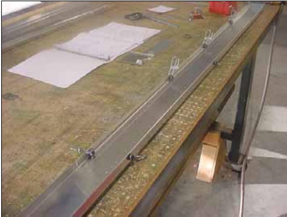
6T1-7HD clamped to the bottom flange.
