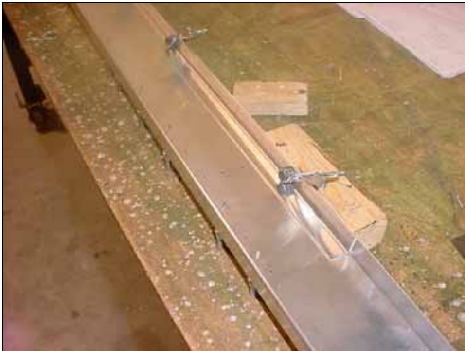
6T1-7HD clamped to the bottom flange.
