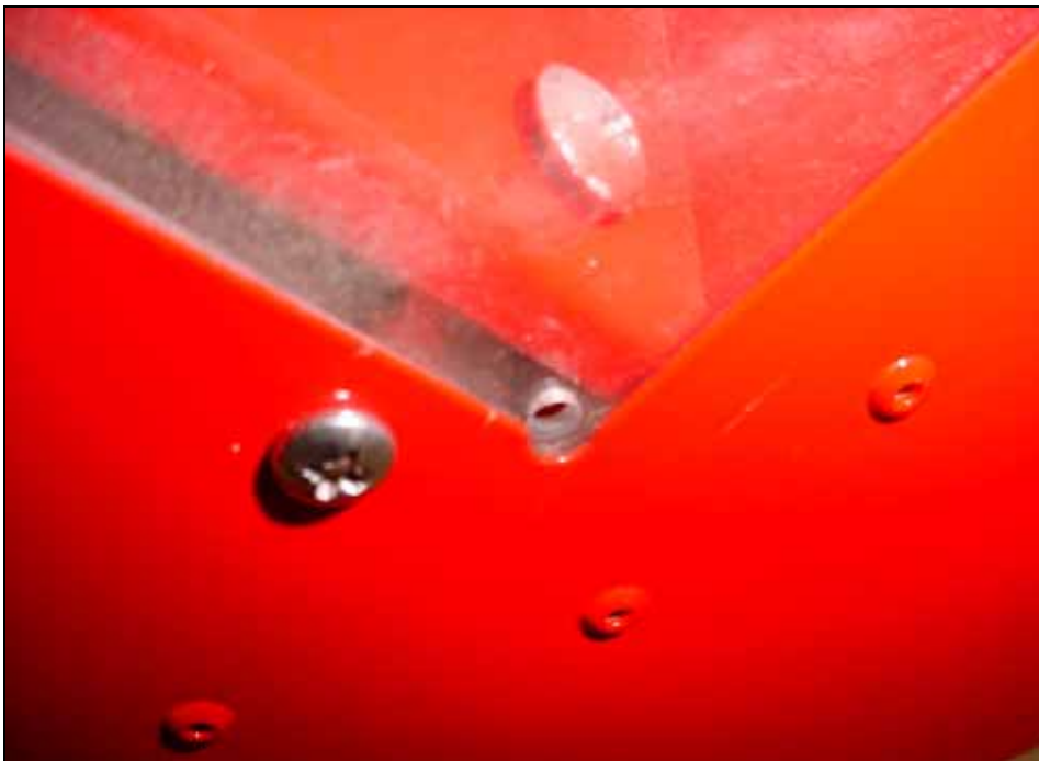
1/8" hole on the bottom of the lens (to help prevent moisture or due build up when the aircraft spends the night outdoors).
