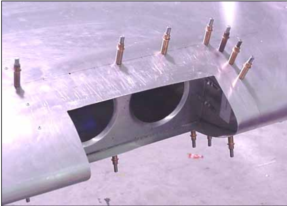
Position the landing light reinforcement assembly against the side of Nose Rib #7, 4 RIVETS A4
