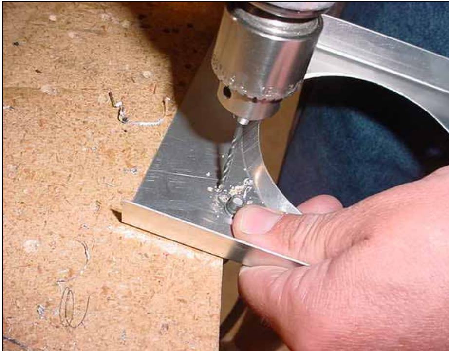
#20 drill bit. Back drill through the nutplate.
