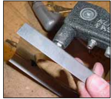
With A3 rivets, rivet the nutplate to the channel.
