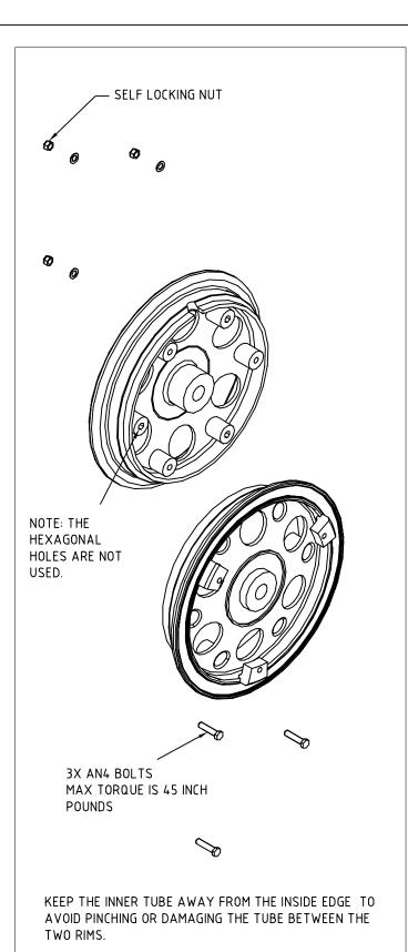
CAUTION: TO PREVENT INJURIES, WAIT TO INFLATE THE TIRE UNTIL AFTER THE THE WHEEL IS SECURELY BOLTED TO THE GEAR ASSEMBLY: MORE THAN NORMAL OPERATING PRESSURE IS REQUIRED TO BEAD THE TIRE TO THE RIM – TO BRING THE EDGE OF THE TIRE UP AGAINST THE WHEEL RIM.
