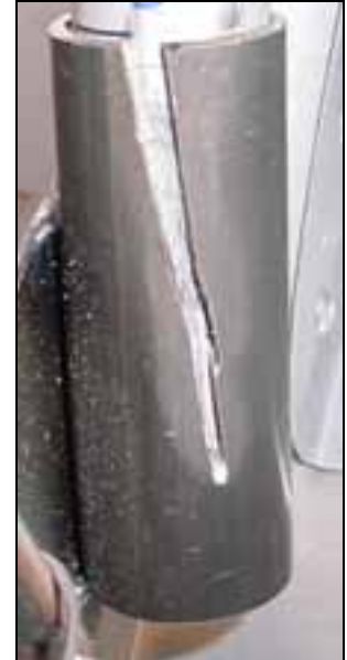
Photo of right side. Insert the tube frame in the 7/8" tube. Use a rubber mallet to drive the steel tube over the canopy tube.
