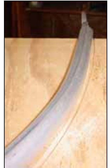
Line around the tube frame on the plywood.
