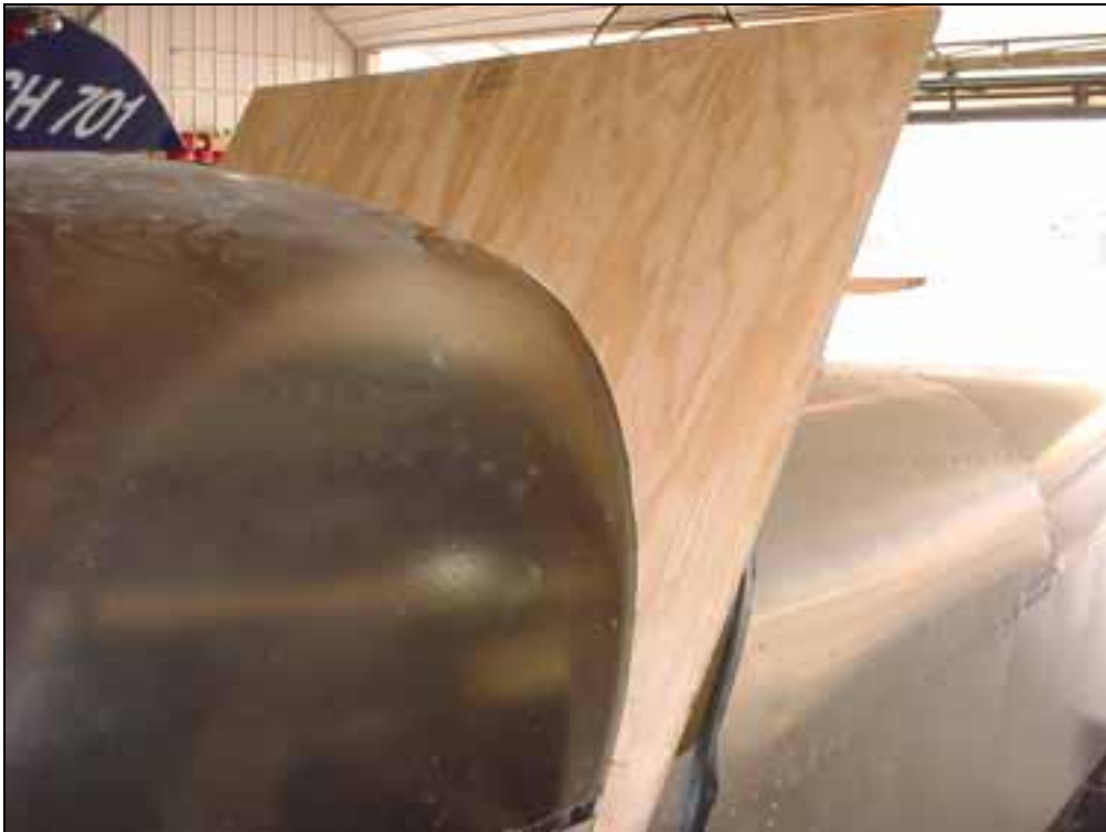
Mark the bottom of the canopy side frame on the template, left and right.
