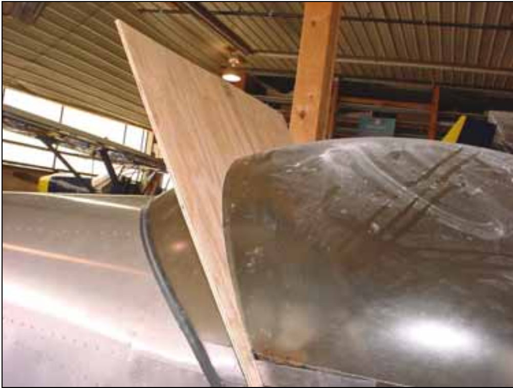
Trial fit. Line up center lines.
