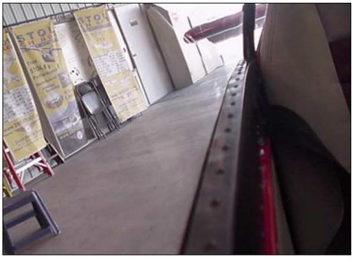
Stretch the top flange of the inside flashing to follow the curvature of the fuselage.
