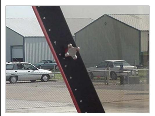
The top flange of the inside flashing will be cut later to clear the canopy tube frames.
