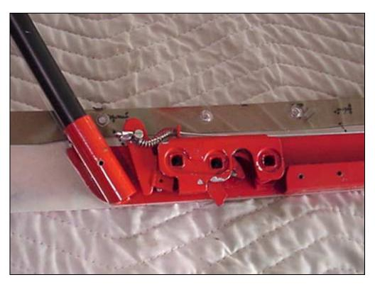
Trial test, insert the Rear tube frame inside the welded 7/8" tube at the back of the canopy side frame. The Tube Frame is too long if the canopy is raised off the fuselage.
