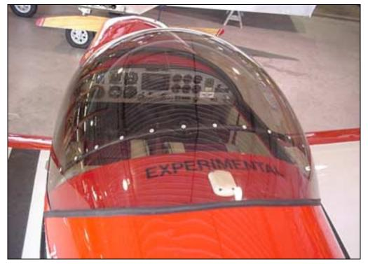
Drill and Cleco through the canopy bubble into the Rear Bent Tube Frame. Use a new (sharp) #40 drill bit.
