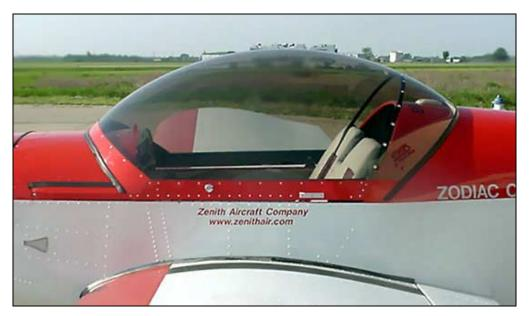
Position the canopy fore and aft: the front bottom corner is in line with the instrument panel. Check: Look at the canopy on profile to find the highest point for maximum headroom.
