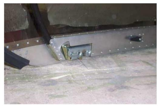
Alternative: larger cutout on inside flashing 6C3-5 to make room for the latch
