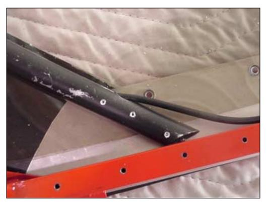
(Photo of right side showing the flexible cable housing to connect the right latch to the canopy open handle mounted on the left side).
