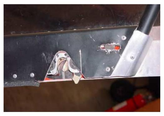
COMMENT: pushing the bottom portion of the lever extension back can also open the latch. Cut off the bottom edge of the flashing (inside and outside) to reach in with a screwdriver. A bend angle with 3 rivets can be used to close the gap between the aft edge of the inside flashing with rear canopy frame.
