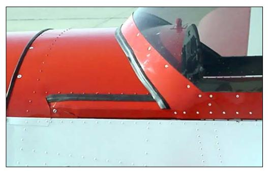
Taper the front end of the cover to avoid interference with the longerons when the canopy is in the open position. The front of the cover is inside the Forward Top Skin 6C1-4
