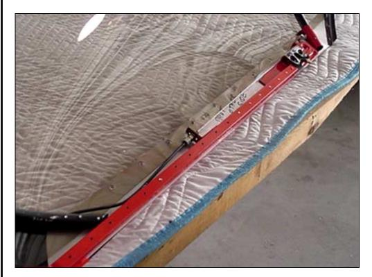
With a grease pencil Trace along the top edge of the outside flashing to mark a line on the canopy bubble.
