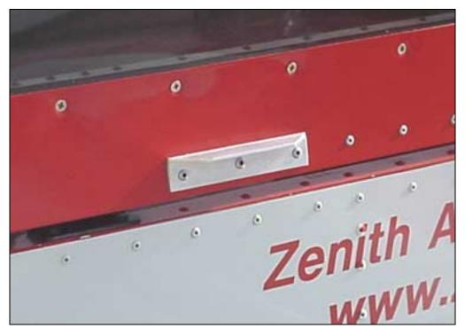
Mark the rivet line along the bottom of the outside flashing, identify the no rivet zone at the front for the gas spring, and at the back for the Handle and latch. Layout the rivet pitch.
