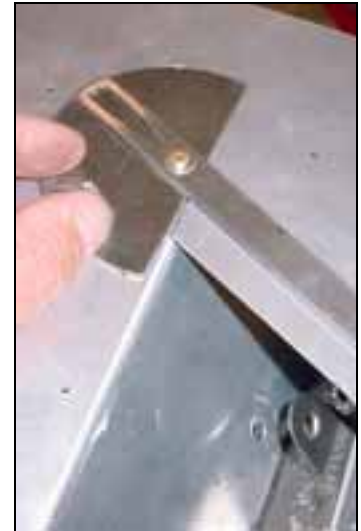
66 degrees. Cutout. For now leave the cutout at the front oversized. It will be trimmed aft the side cover 6C3-6 is installed.
