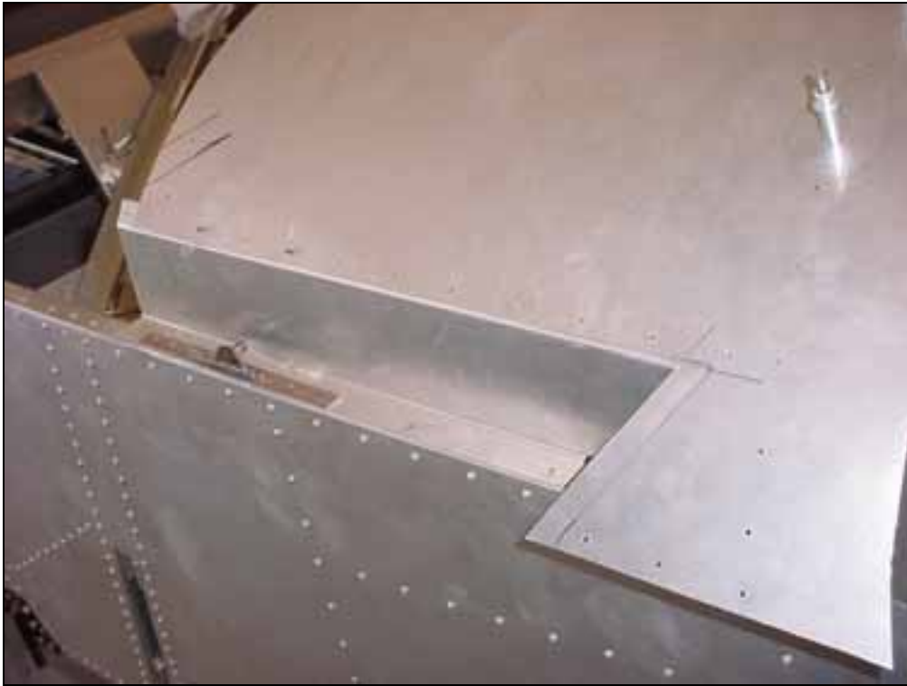
Drill and cleco the top flange of the panel side angle 6C1-1 to the forward top skin 6C1-4
