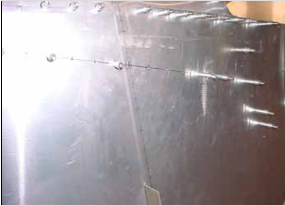
Layout the rivet line through the seat back side channel 6B16-3
