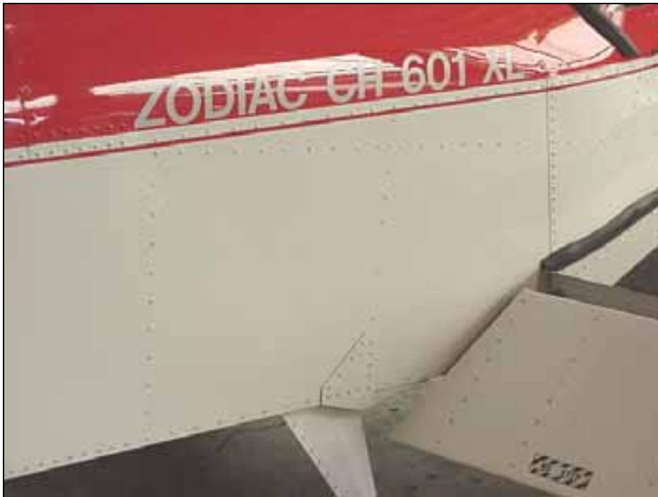
Detail of the longeron splice. Ref. 6-B-14
