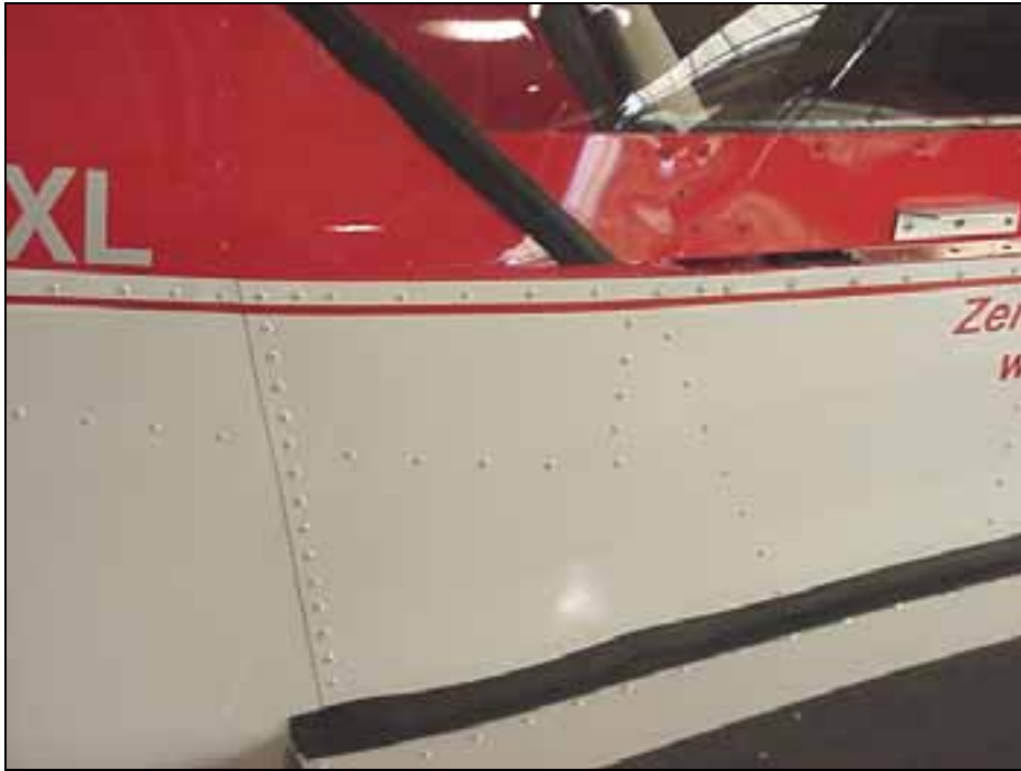
Detail of aft edge of the forward side skin 6B11-2.
