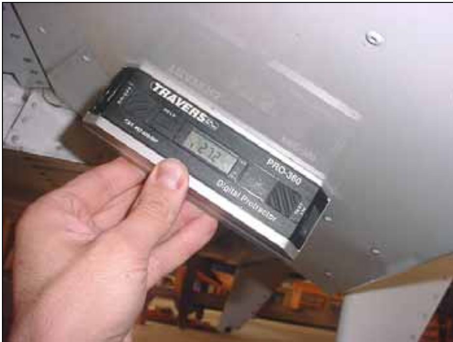
Flaps down, approximately 27 degrees (flap actuator fully extended on the worm gear).
