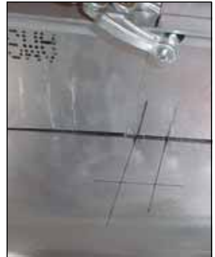
Transfer the marks from the side skin to the bottom skin. Ref page 4 of 12 bottom photo section 6-B-16A
