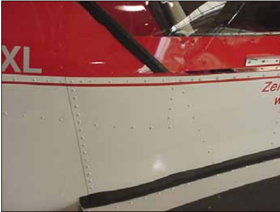
Detail of rivets lines on demo aircraft.
