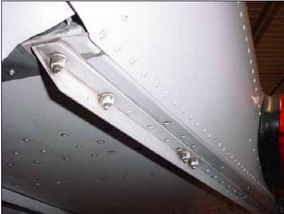
Detail of the bottom rivet line in the side skin
