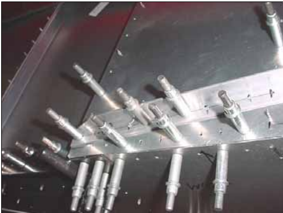
The last (aft) rivet in the outboard rivet line. Approximately 45mm to the aft edge of the cabin floor skin 6B10-1
