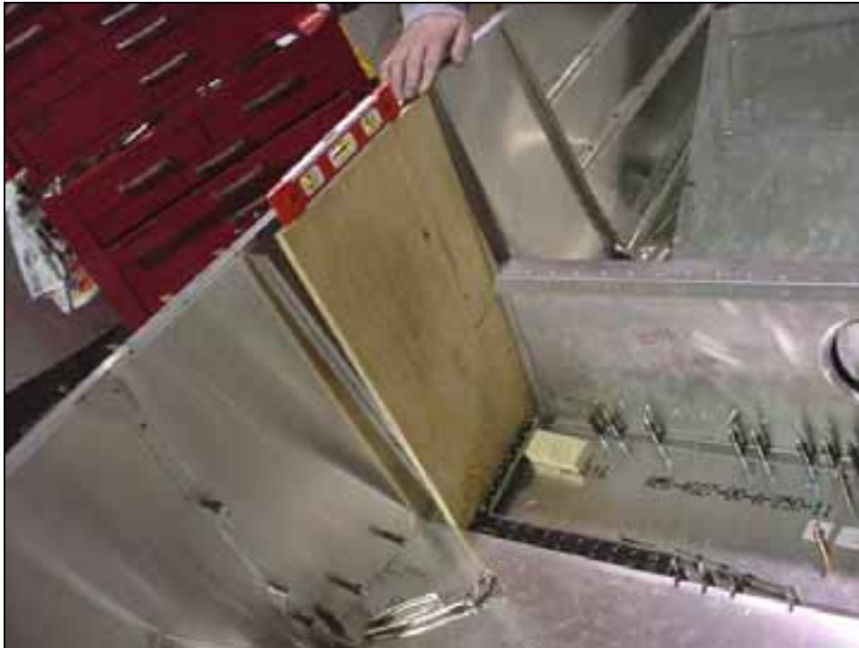
Rear view of left side. Position the diagonal side of the template against the Upright 6B13-1.
