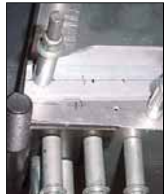
The last (aft) rivet in the outboard rivet line. Approximately 45mm to the aft edge of the cabin floor skin 6B10-1
