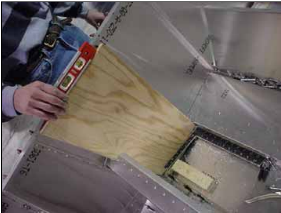
Photo of left side. The Spar is at 9 degrees to the Longerons.
