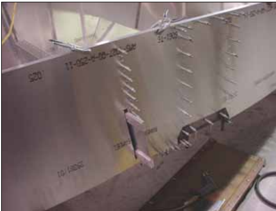
Lay out the rivet line, set the pitch. Drill and Cleco.
