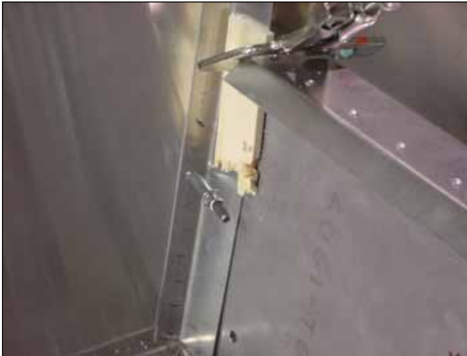
Rear view of right side. Clamp the top of the wing attachment 6B13-1 to the side skin.
