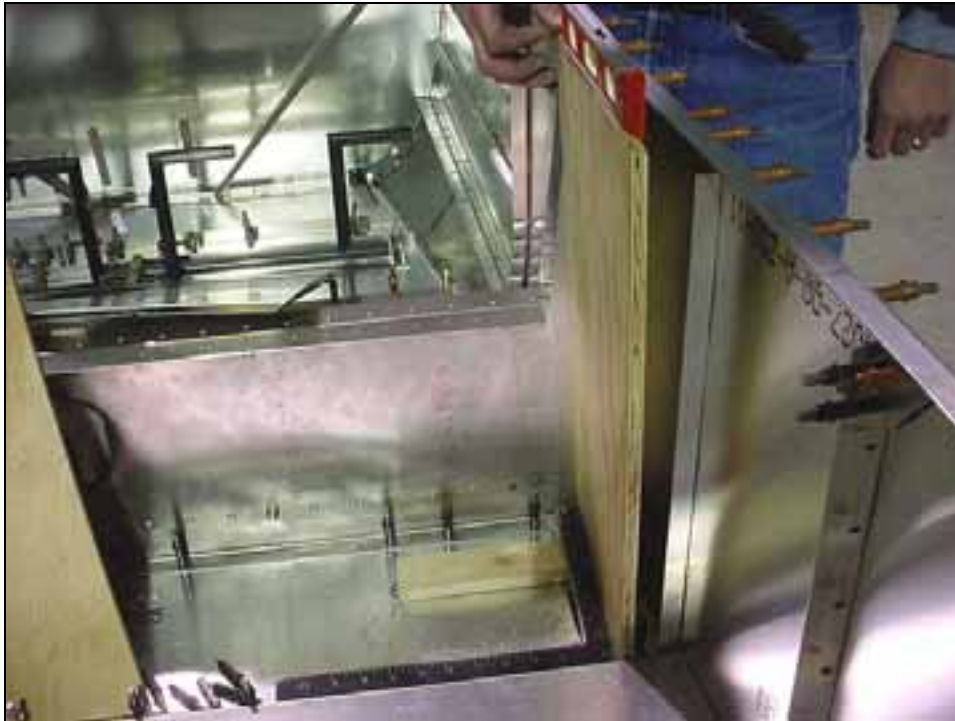
Rear view of right side. Clamp the top of the wing attachment 6B13-1 to the side skin.
