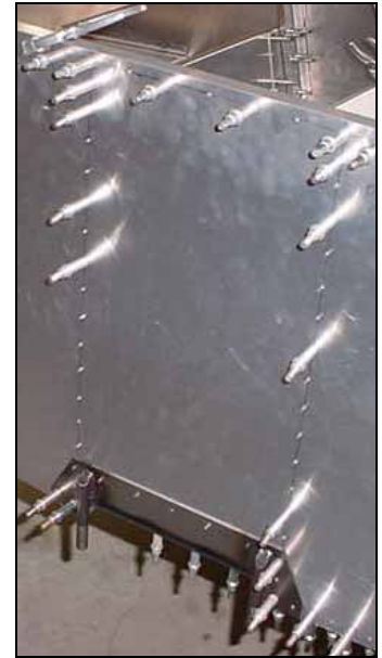
Rivet lines on outboard side of skin.
