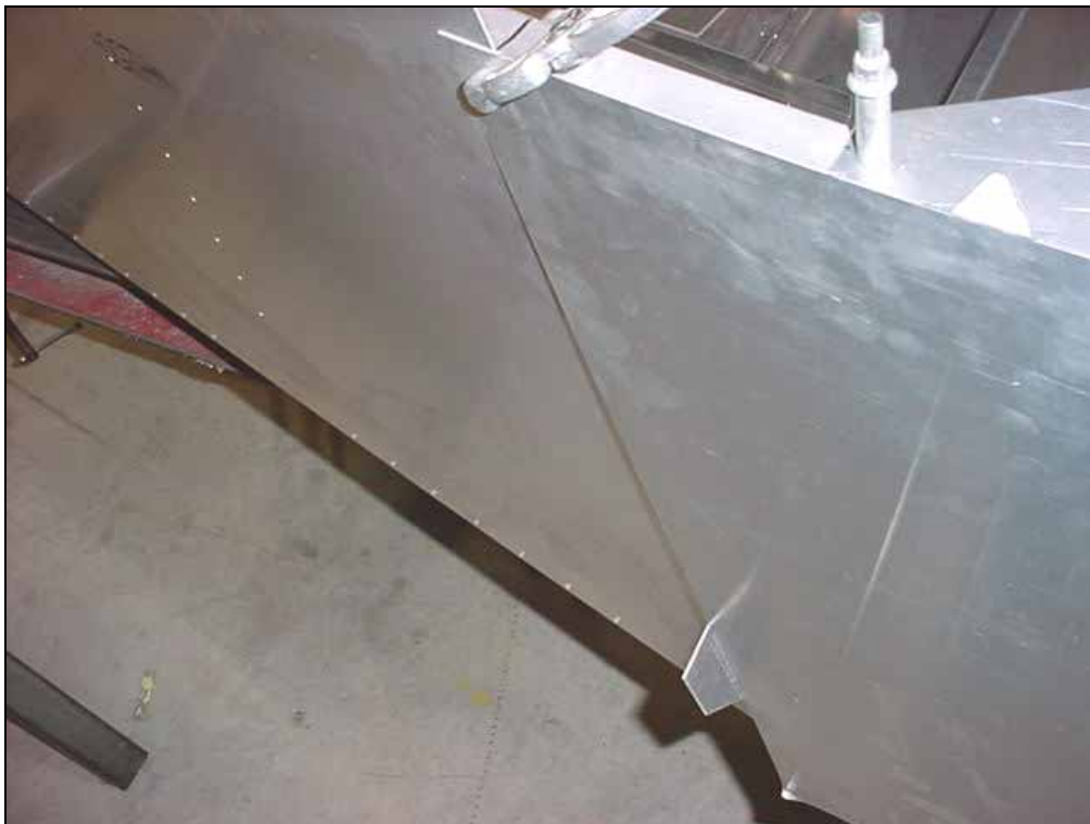
Clamp the top edge of the skin flush with the longeron.
