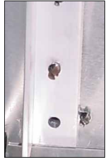
From inside the fuselage, drill the bottom bolt hole in the uprights 6B11-3
