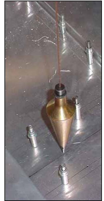
Aircraft center line on cabin floor.
