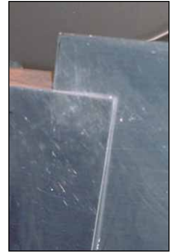
Detail of left overlap. Skins overlapped approximately 24mm
