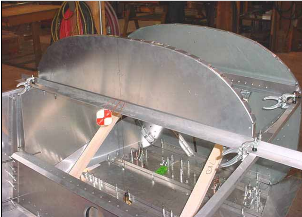
Plumb center lines.
