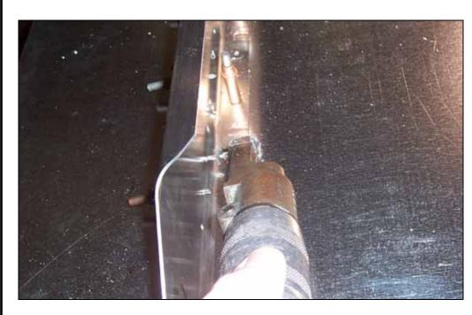
**Note:** Be careful that the Drill Chuck does not damage the Firewall Top Stiffener or the Firewall when drilling.
