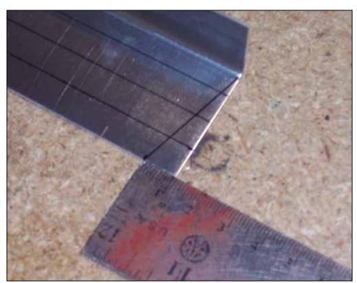
Mark a line from the start of the bend radius to a point 10mm from the end of the Firewall Side Stiffener. Trim the Firewall Side Stiffener along this line.
