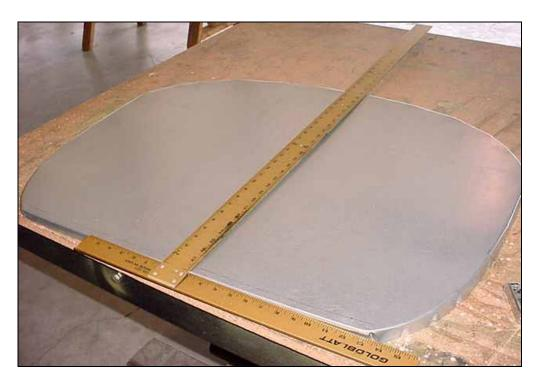
**Check:** the center line is square to the bottom of the firewall.
