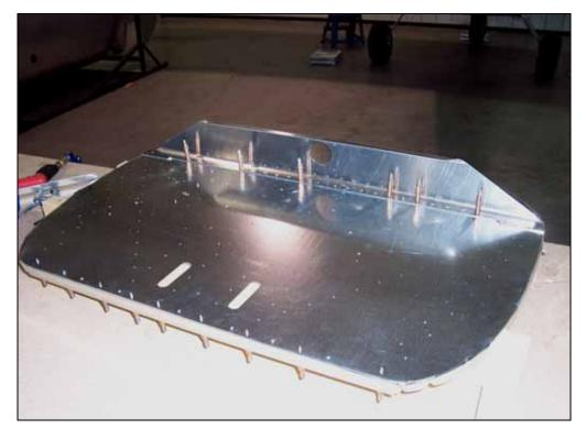
Cleco the Firewall Top Stiffener to the Firewall. Expand the predrilled holes first with a #30 drill then to #20, Cleco every other hole as you drill.
