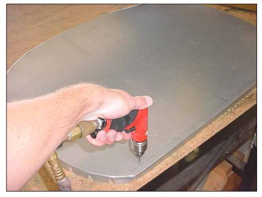
Back drill through the predrilled holes in the Firewall through the Firewall Bottom Stiffener (flange that overlaps firewall, do not drill bottom flange).
