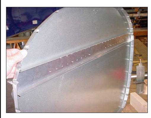
**P/N:** 6B7-2 Firewall Reinforcement
