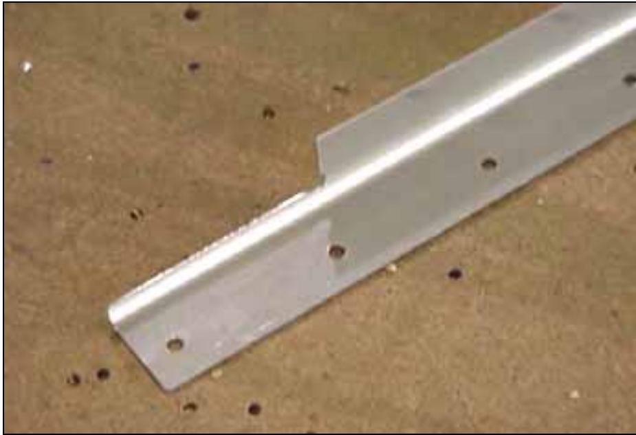
Location of the L angle in front of the cable outlet fairing
