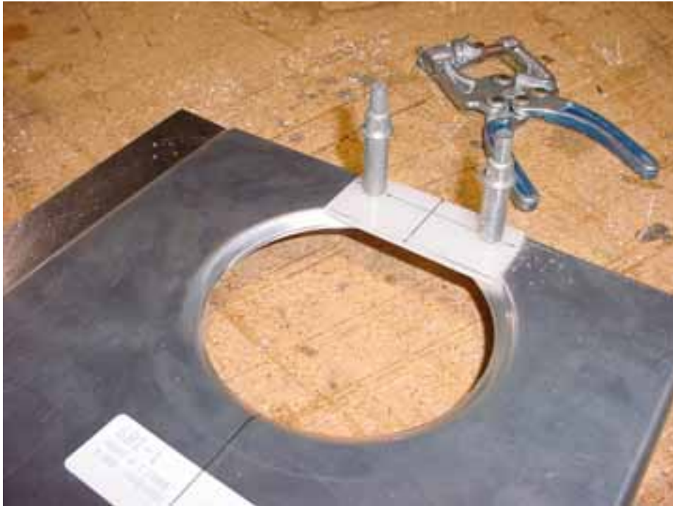
Cable Fairlead (1/8 plastic material). Positioned on the front side of the Front H.T. Frame 6B1-1. Back drill to the H.T frame.
