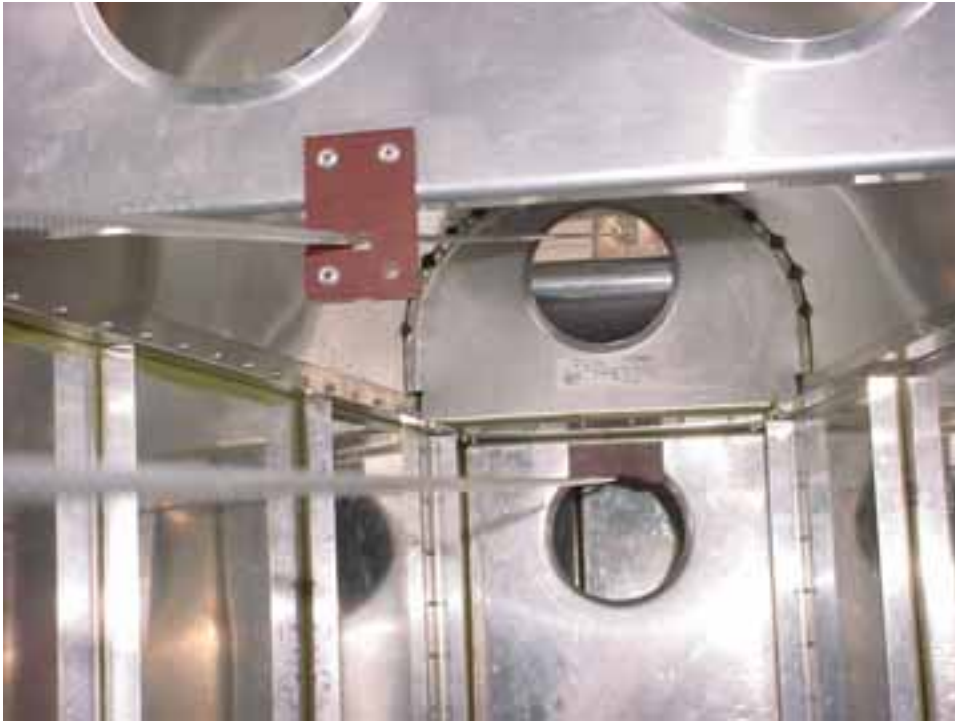
Photo showing the elevator cable and fairleads.
