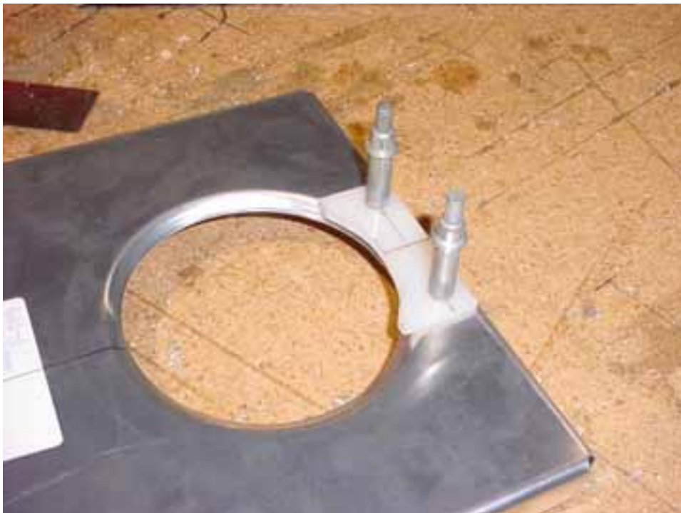
Contour the bottom of the fairlead to match the curvature of lighting hole.
