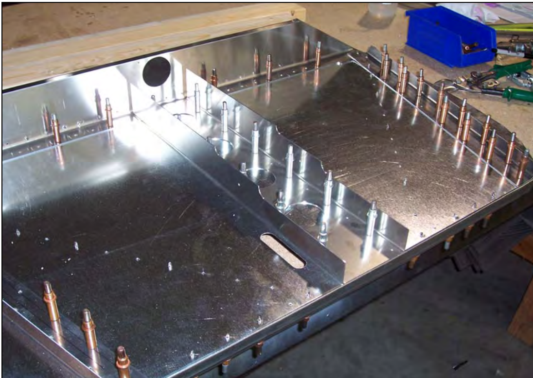
P/N: 6B8-7 Center Firewall Stiffener
