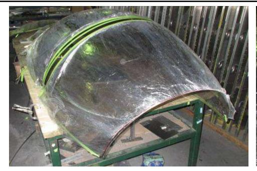
Remove the bubble from the fuselage and cut.
