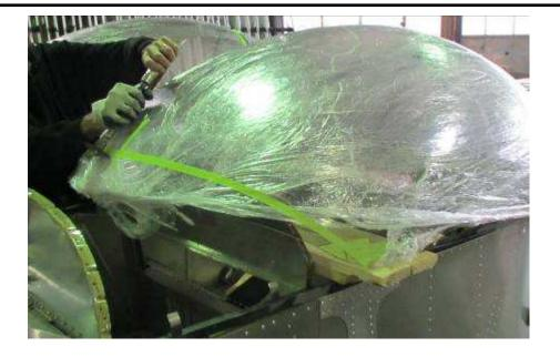
To cut the canopy on the fuselage, raise the canopy with a board across the fuselage.
