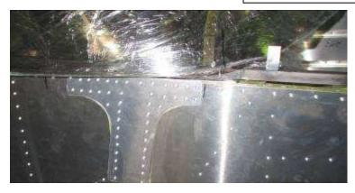
Mark the location of the weld with a vertical line. Mark the cut even with the top of the canopy side frame
