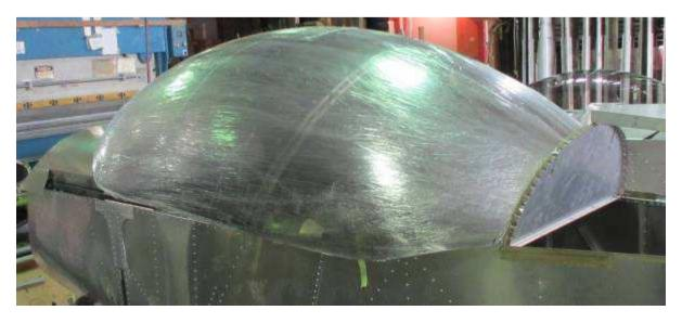
Let the back the bubble overhang on the outside of the fuselage.
