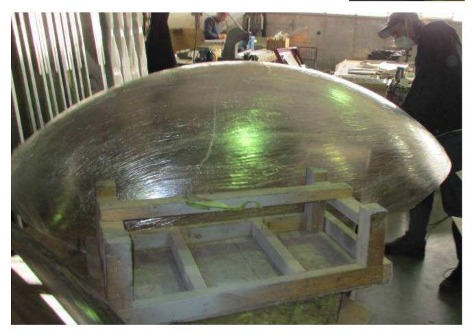
Support the sides of the bubble to keep it from spreading open.
