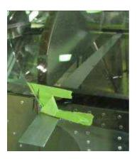
Slide a strip across fuselage to the support the front edge of the canopy
