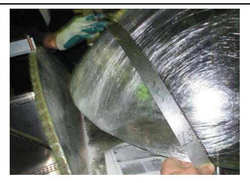
REAR – measure up 290mm along CL and 520 from CL along the bottom edge (left and right). Connect the 3 points with a flexible straight edge.
