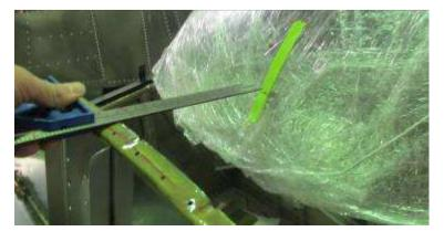
Push the left and right sides of the bubble against the side frame, sight across the firewall and instrument panel and mark a point approximately 40mm below the top skin on the aircraft center line.
