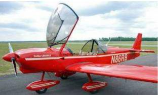
With the canopy 190mm behind the firewall, it will open with adequate clearance with the top skin
