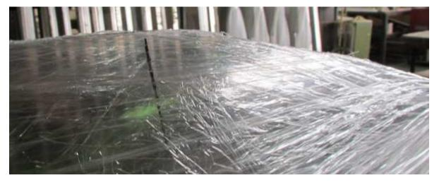
Rear right mark. The shorter perimeter distance is the front. When looking at the bubble from the side, note the front bottom edge is cut on a steeper angle than the slope at the rear.
