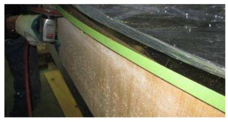
Trim the sides even with the top of the fuselage.
