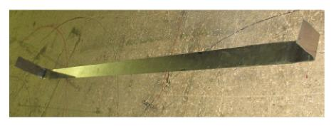
Support strip (positioned on the cabin-side of the instrument panel) to keep the front edges of the bubble even with top of the fuselage sides.
