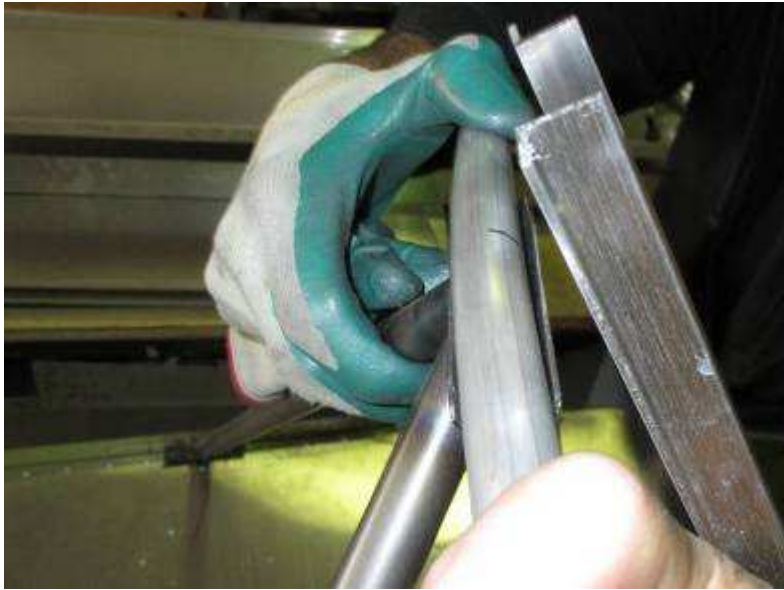
Reassemble and cleco the base of the roll bar to the fuselage.
