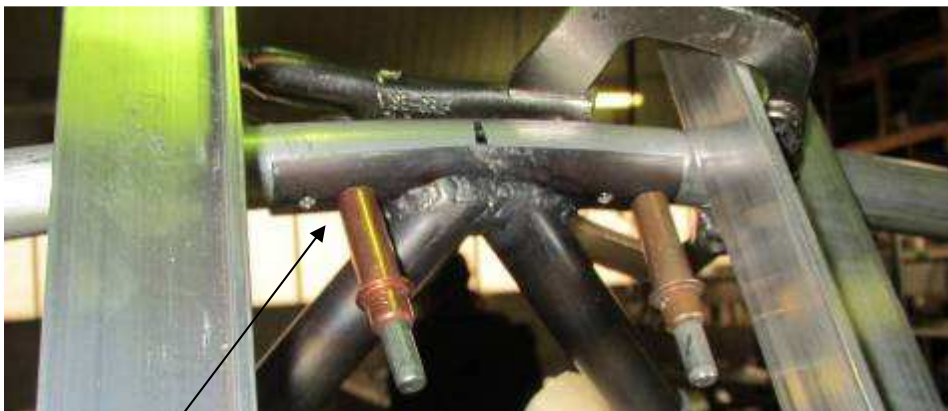
Tape the tube to the roll bar (wait to drill the tube until after the front canopy is installed).
