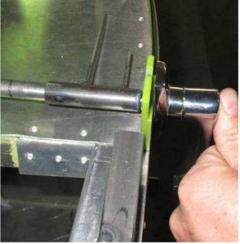
Position the assembly on top of the fuselage. Check for approximately equal distance from the left and right O/B tube to the reference line.
