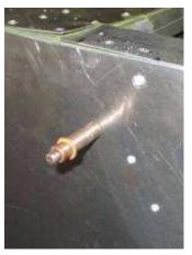
From the inside, drill the front bottom hole in the bearing. Cleco from the outside.
