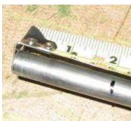
Mark the lines from each end of the MAIN CANOPY LOCK TUBE 65C5-1
