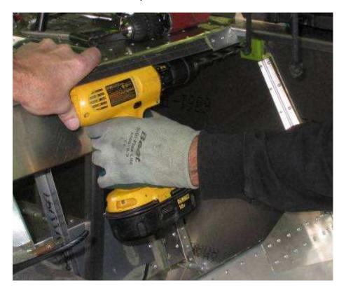
Position the handle and drill the front hole through the bearing.
