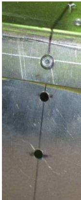
Open up with a 3/4" hole saw or uni-bit
