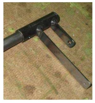
25mm overlap - insert the ends on the tube - make sure there are no burrs inside the tubes -
