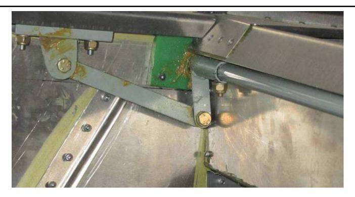
Paint the steel parts and re-assemble with bolts.
