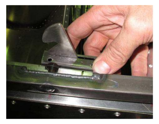
Open the latch and mark the aft edge. The length of the slot is between the closed and open position.
