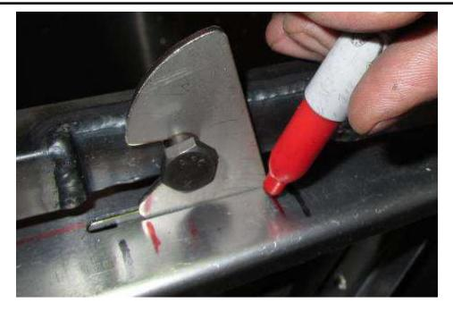
Check that the slot is long enough to swing the latch open.
