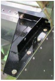
NOTE: The hinge hole is drilled square to the fuselage sides.
