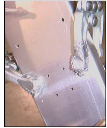
Clamp the rib to the spar. Use the toggle clamps.
