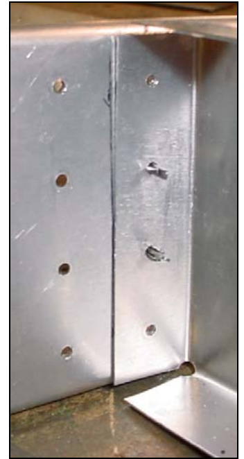
65T4-1 Drill and Cleco the nose rib to the spar.
