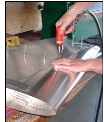
Start drilling from the center, working towards each end. Drill both sides.
