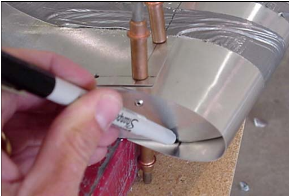
Start drilling from the center, working towards each end. Drill both sides.
